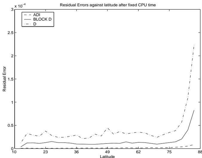
Figure 4: Latitudinal variance in convergence for Limited Area Helmholtz problem with Diagonal, Block and ADI preconditioners. Northern boundary at  $88^\circ$ ,  $h = 1^\circ$ ,  $k = 0.01$ .
